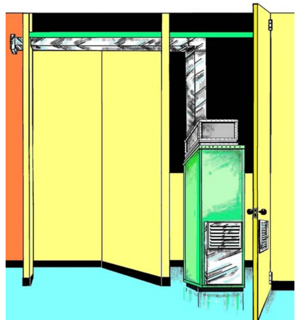
New updraft furnace with new duct trunk line.
